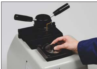
Back-and-forth slide and flip motion mold enclosure provides easy access to mounts
